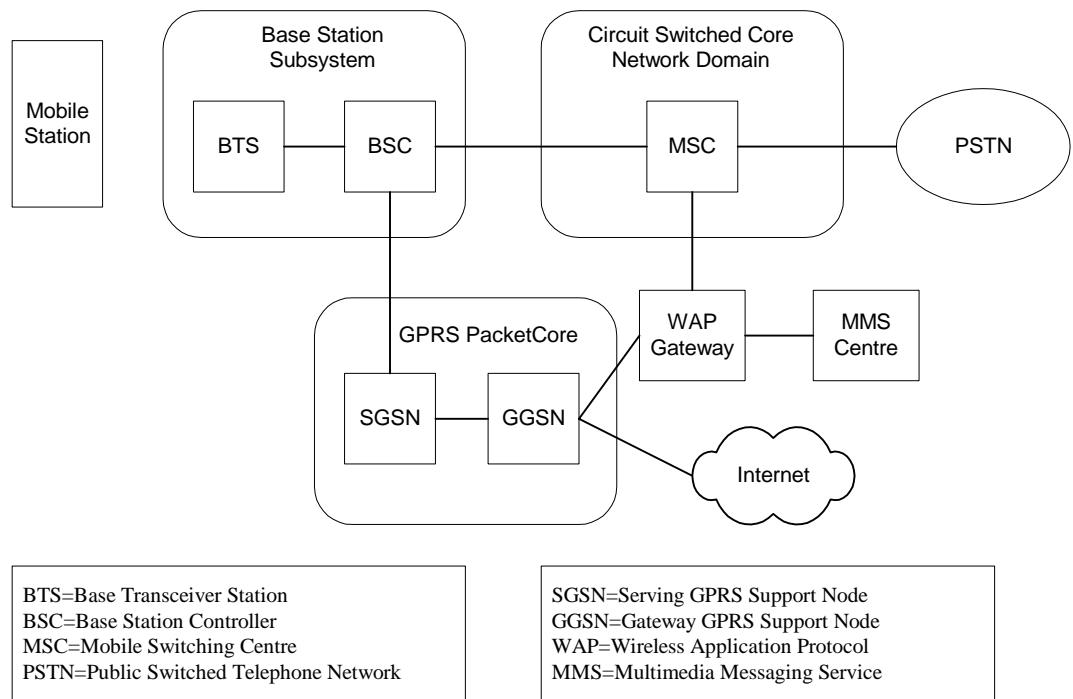
**Figure 2.4 Architecture of WAP implementation of MMS.**
