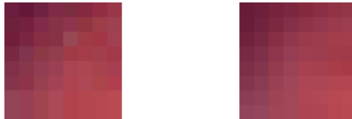
Figure 4.3 The last 8x8 block of the Lena image before and after JPEG coding.
